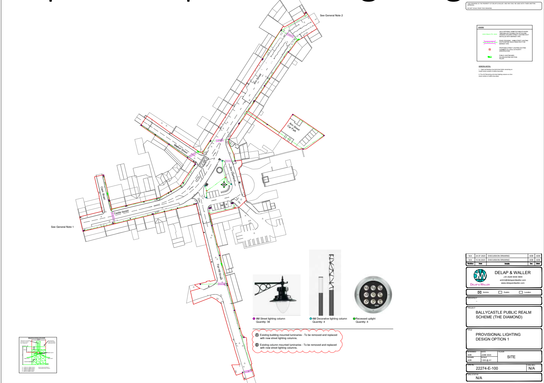
Technical drawings of The Diamond showing existing and proposed lighting locations (option 1).
