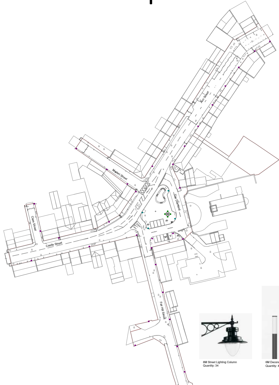
Technical drawings of The Diamond improvements (option 2) showing lighting designs.
