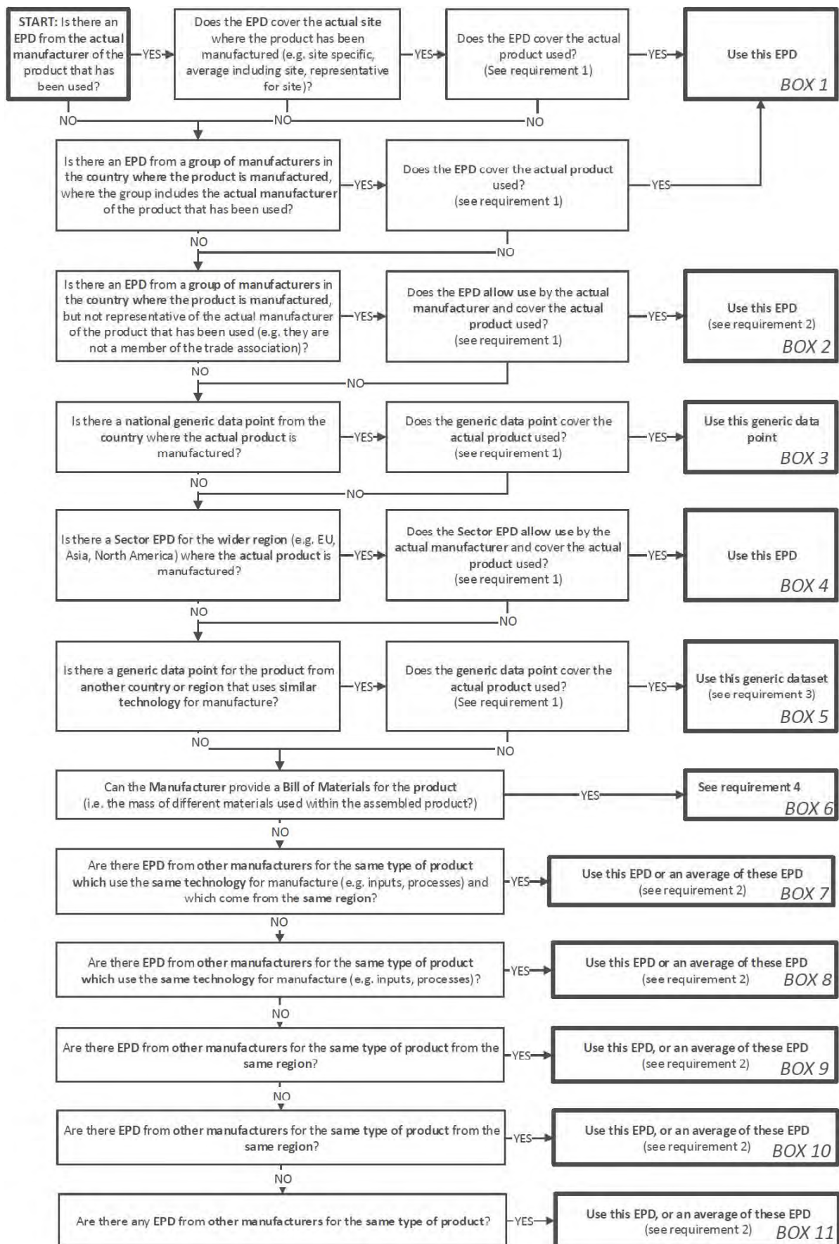
Figure 8 Carbon data selection flowchart, products/materials/systems life cycle module A1-A3
