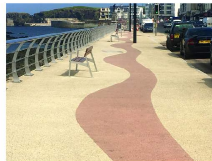
Typical view of mixed exposed concrete aggregate to be used, as identified within Play Area
